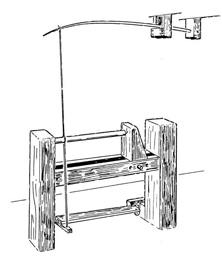
The spring pole lathe is thought to have been the next development in the evolution of machine tools. It was operated by the artisan's foot and left both hands free to handle the cutting tool.
