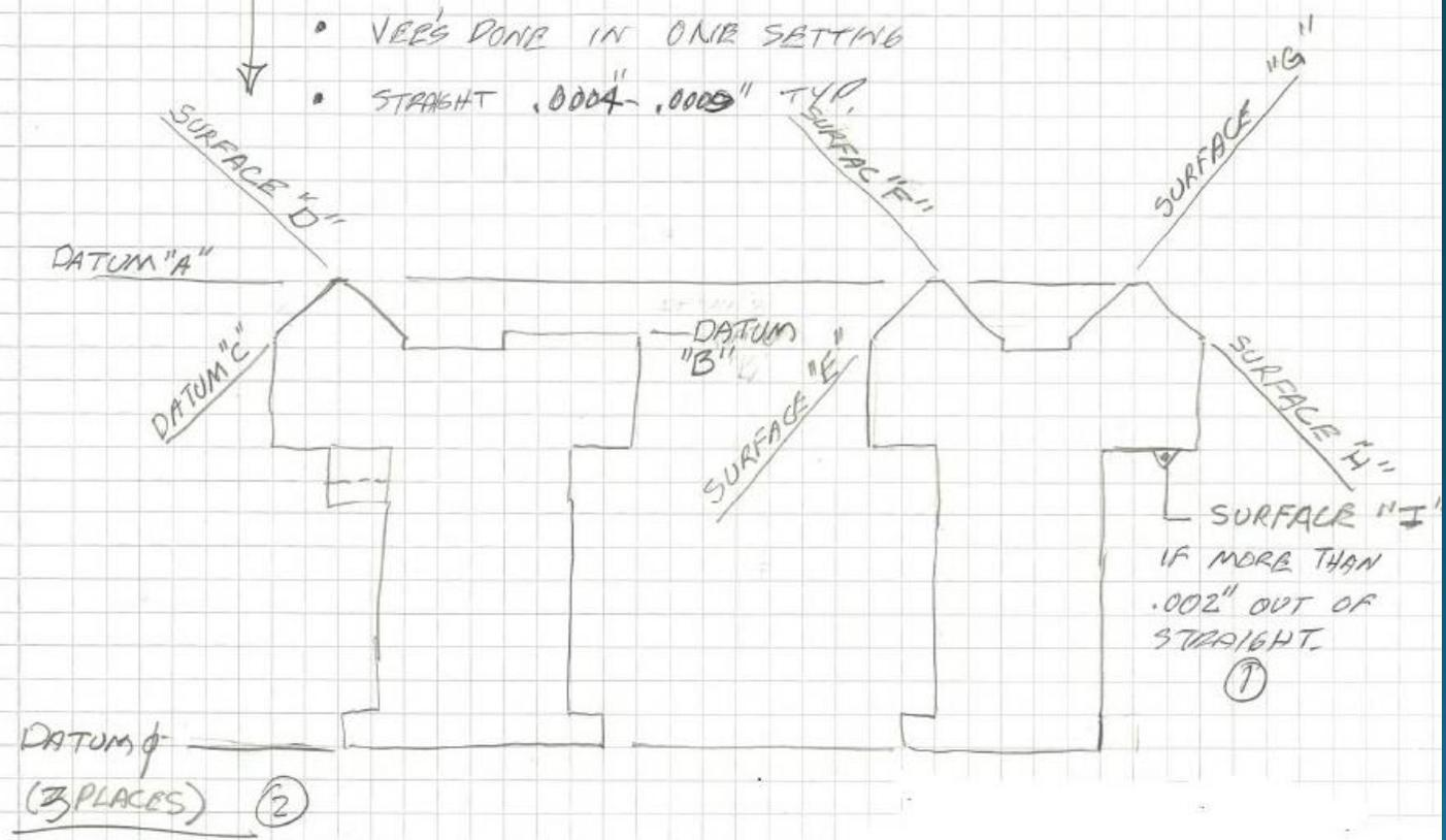
The key surfaces to be ground on the bed as conveyed to the grinding house.
