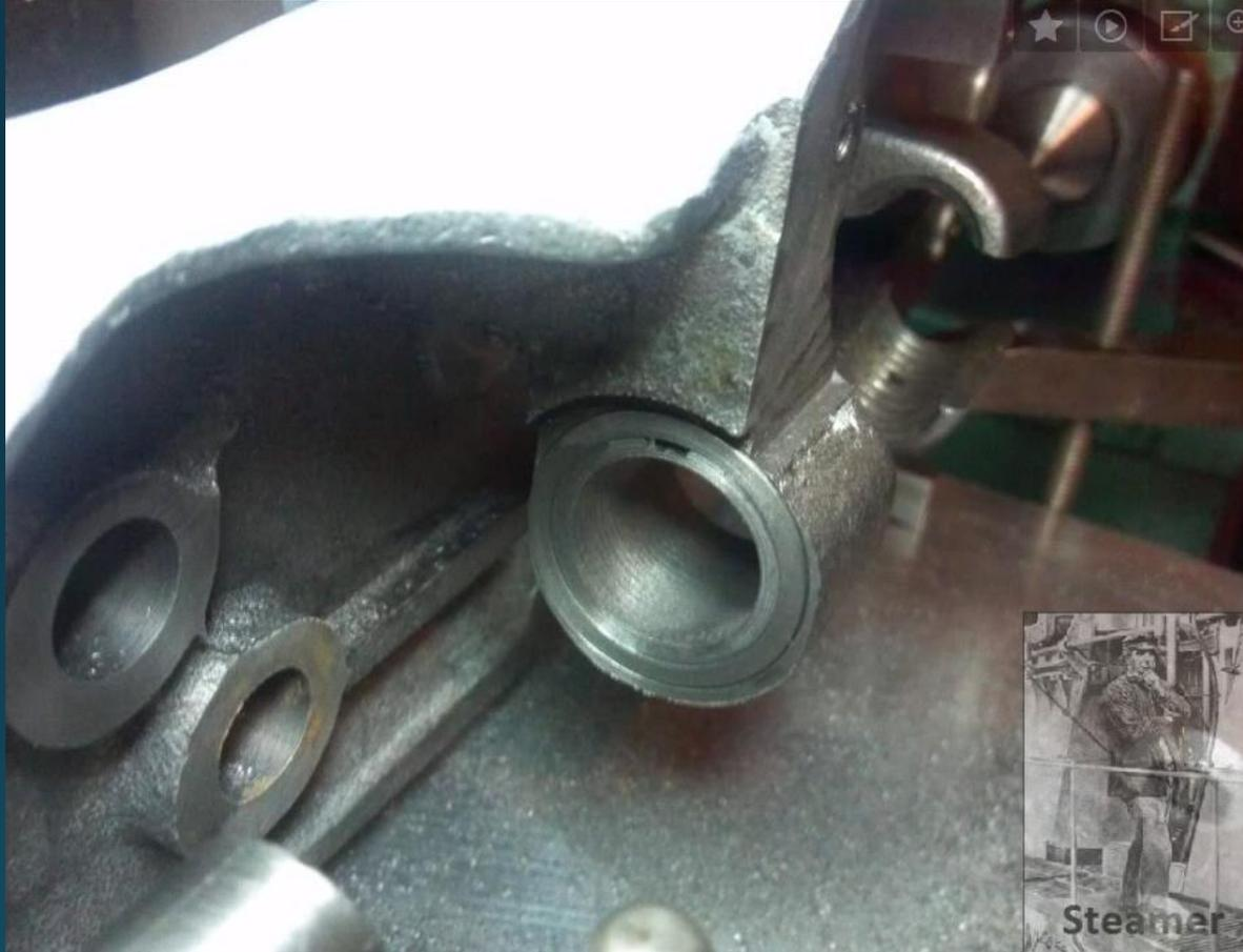
Bushing installed just prior to boring the bushing to size
