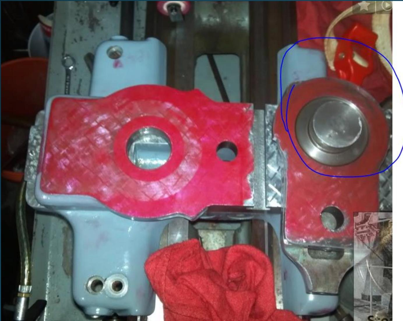
Notice the un marked area near the Nose of the compound. This is wear as A result of chips getting under the Compound and wearing away the surface
