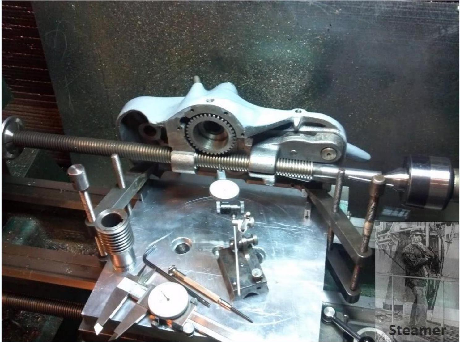
Set up on the boring table
