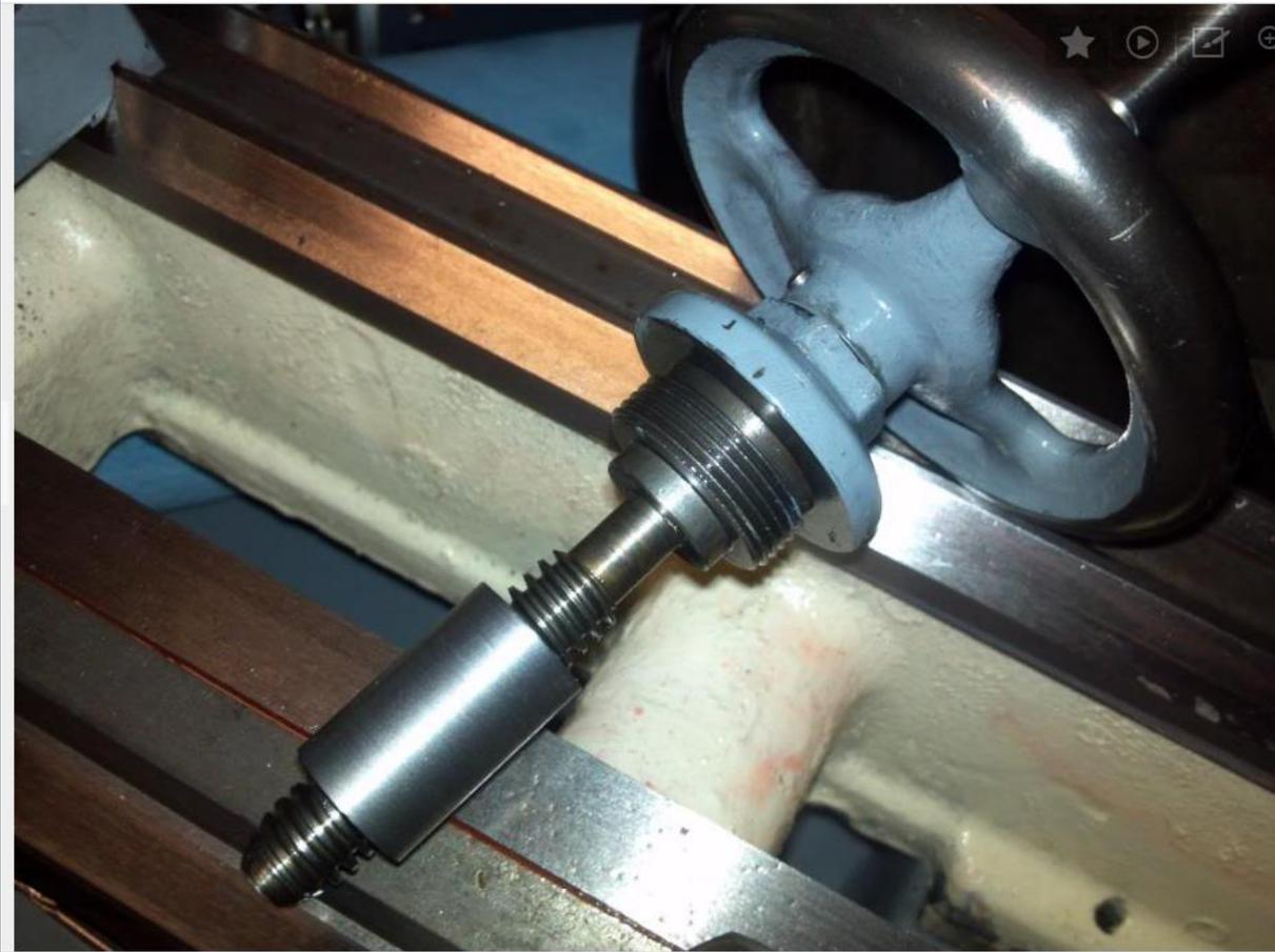
The old quill had the nut pinned in place. I decided To machine the quill and leave just this Remnent as the nut for the new quill. I then installed It into position with Loctite. It worked quite well!
