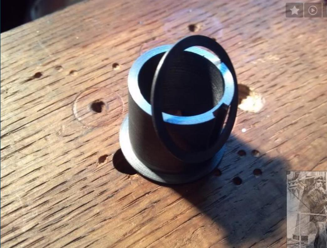
I machined a bushing to a close fit with the Worm gear, and a nominal fit with the new Hole I was going to bore. You will notice the Slot on the OD. This bushing was then loctited Into the new housing bore, and then bored to size. When to size, the slot was open. Then a standard wick could be fitted in place.
